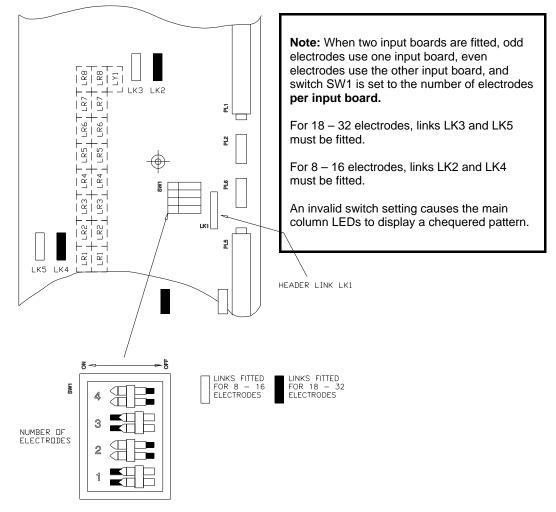
Figure 2.5- Location of display board links LK1 to LK5 & switch SW1 with configuration details
